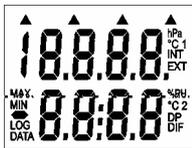
Switch ON the instrument by pressing ON/OFF key. After switching ON the instrument all symbols on the LCD are displayed. If the ON/OFF key is being held pressed, all LCD symbols are displayed till the key is released. In usual operation instrument then starts the measurement mode and actual measured values are displayed.
