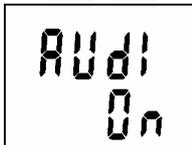
This item indicates if audio signaling of alarm indication is switched on (On) or switched off (OFF). Press ENTER key to change actual setting. Notice: if the battery voltage is low, audio indication is out of operation to reduce current consumption independently on this selection.
