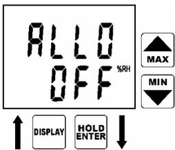
Then you are offered to set alarm of other input value (here relative humidity). The procedure is the same as the above temperature limit setting. Alarm activation of each value can be disabled by setting lower alarm limit of the desired value up to its maximum. This is indicated by OFF reading at the position of numeric value. Value of upper limit of the same alarm is indifferent.
