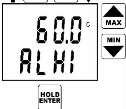
Reading ALHI indicates adjusted upper limit of the same alarm (here air temperature). Set the desired value in the same way as in above lower limit. If needed it is possible to get back to lower limit setting of the same alarm by pressing DISPLAY key. Press ENTER key to confirm new upper limit.
