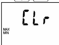
Clearing of minimum and maximum memory of all values. Memory is cleared after pressing ENTER key. Clearing is confirmed by reading YES on the LCD lower display.
