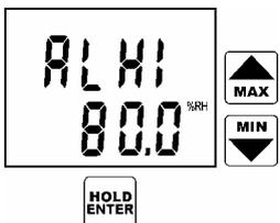
It is possible to leave the alarm setting mode by pressing MENU key. New adjusted limits up to pressing MENU key are stored in memory.
