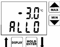
Reading ALLO indicates adjusted lower alarm limit (here air temperature). Set the desired value by means of the arrow keys. Press and hold the arrow key UP to make value increase fast. Press and hold the arrow key DOWN to make value decrease fast. Release the arrow key and press ENTER to confirm new limit.
