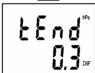
Press DISPLAY key to display pressure tendency (hPa), which is the difference between actual pressure and pressure before 3 hours. If the instrument is not switched ON at least 3 hours, pressure tendency is not available yet and symbol „--„ is display.
